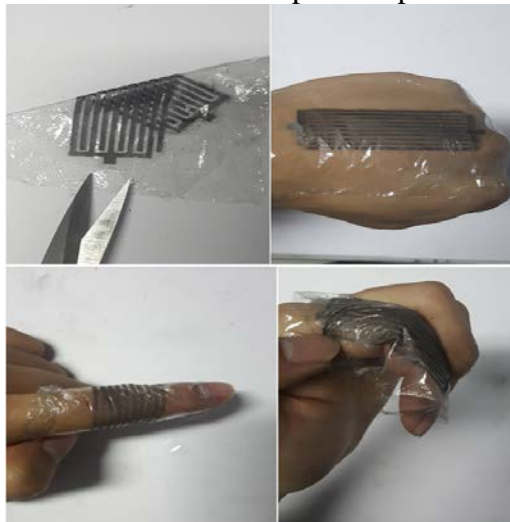
Figure 3. Flexible performance of planar capacitance under physical deformation
